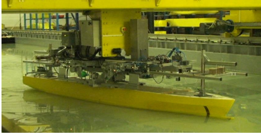
Figure 4.1 Ship model tested in free-running mode.
